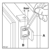
At the end of installation/adjusting, it is necessary to check if the door of the furniture closes properly. Should the lining up of the furniture door be necessary, use the
